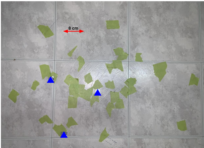
FIG. 3. Map of points of contact with the ground. The location of the three strings are denoted by the blue triangles and the contact point of each drop is recorded with green tape. The length of the red line is 8cm. The paper was held parallel to the tile markings.
