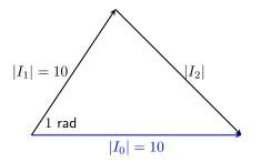
The sum of the two phasors  $I_1 + I_2$  needs to be horizontal (which represents no phase shift), and we can determine this using cosine law:
