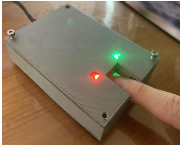
FIG. 6: The final 3D printed prototype in the worker mode. Note that only two screws were installed since we only had access to two screws. The effects of material constraints and our own poor manufacturing devices (not the MyFab printers) are discussed in section IV C .
